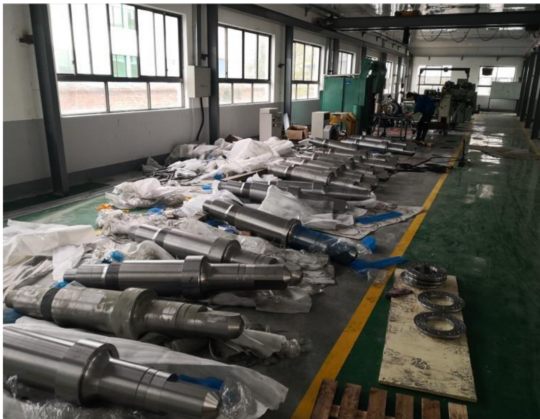
Composite roll components--- steel roll shaft and spacer ring
