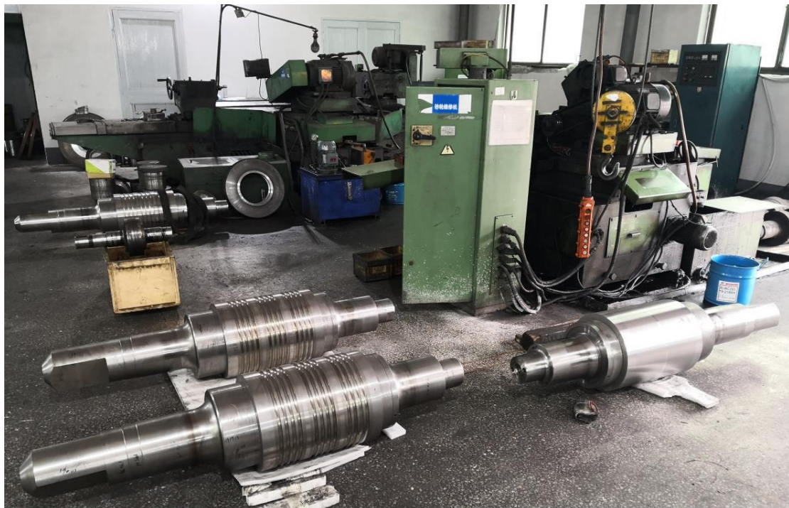
Composite roll finished processing workshop
